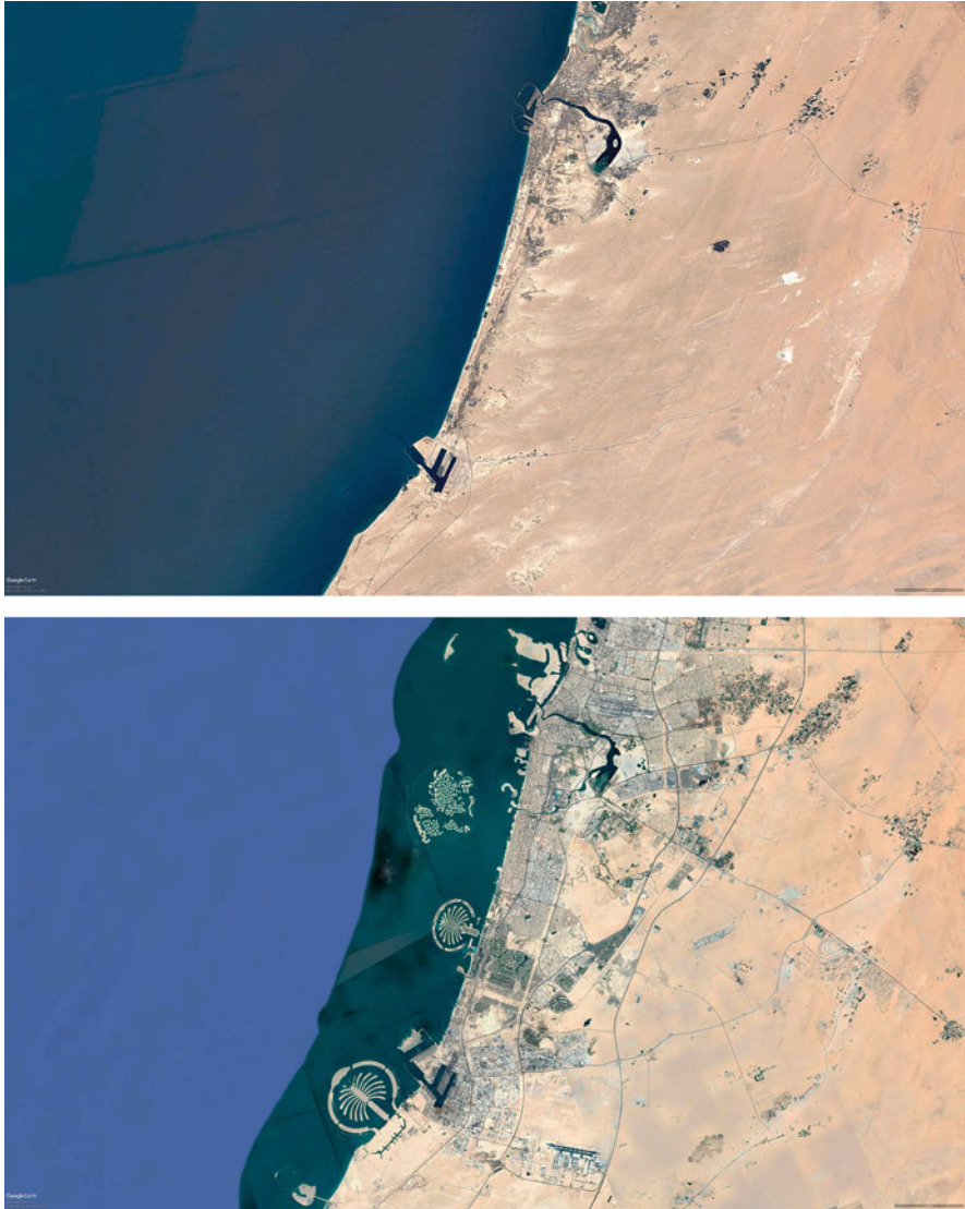
Fig. 3 Comparison of coastal development in Dubai in 1984 (top) and 2018 (bottom), showing the Palm Jebel Ali, Palm Jumeirah and The World offshore developments in addition to coastal reclamation and urban sprawl. Images courtesy of Google Earth
