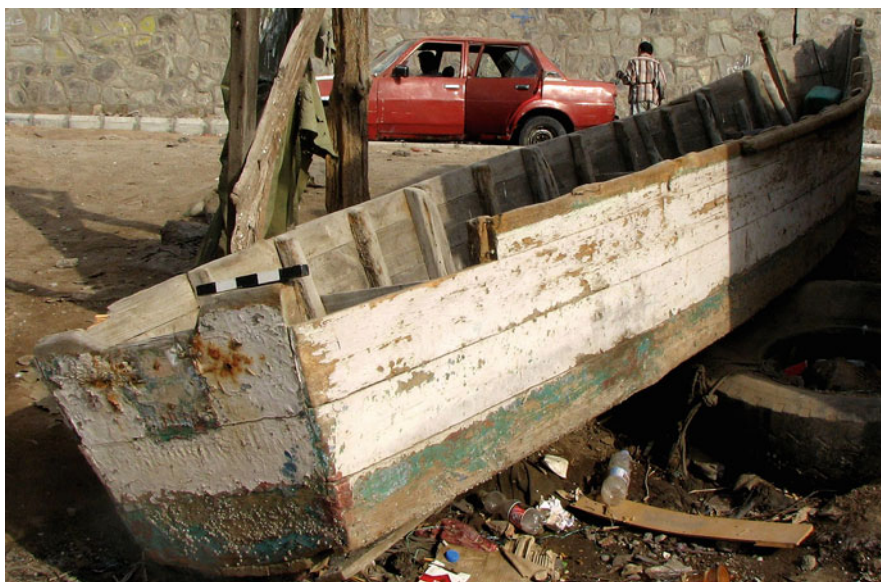
Fig. 42 Very simple planked hūri , Ma'allah, Yemen, 2007, courtesy of John Cooper, England
