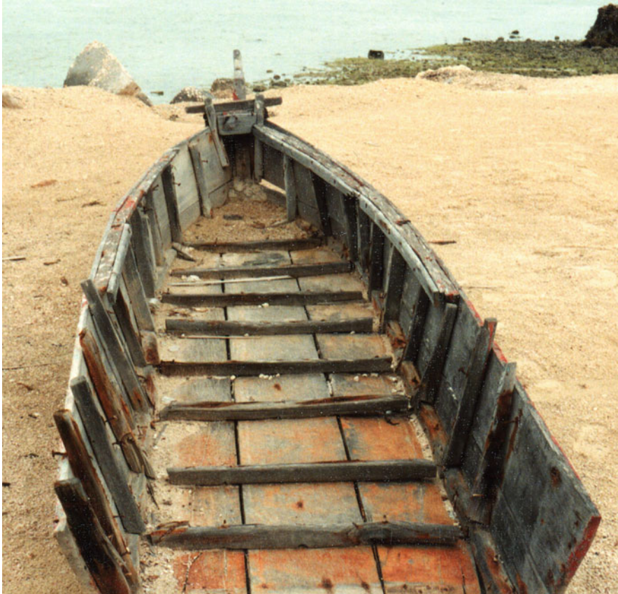
Fig. 18 Flat bottom boat with transom, Al Khor, Qatar, 1997, photo Weismann
