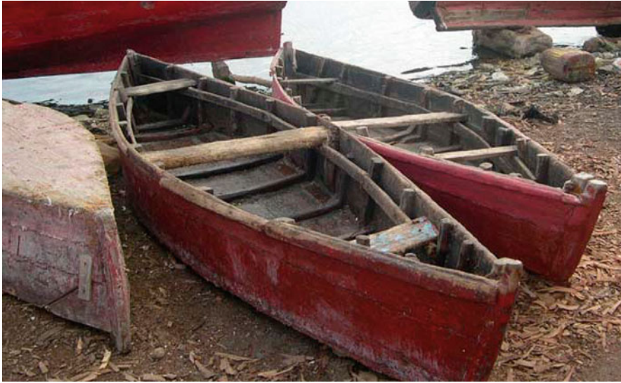
Fig. 44 Small planked flat bottom hūrīs , Suakin 2004, from Agius (2012, 183, detail)
