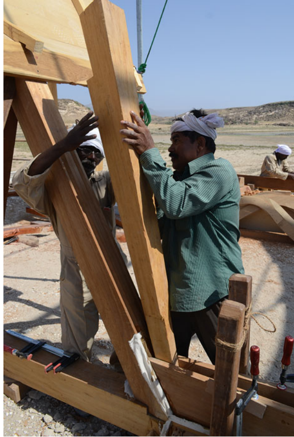
Fig. 4 Setting the internal stern post, sanbūq Dhi'b, Khor Rori 2011, courtesy of Alessandro Ghidoni, England
