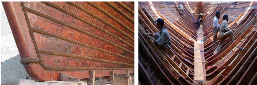
Fig. 11 Plank seams showing wadding on both sides, outside and inside Jewel of Muscat (Image courtesy of Alessandro Ghidoni)
