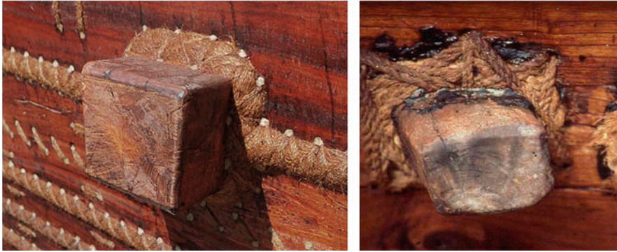
Fig. 10 Sewing of beam ends on Jewel of Muscat (after Belitung shipwreck) and on a twentieth-century battil (Image courtesy of Alessandro Ghidoni)
