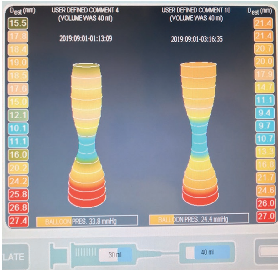
Fig. 8.7 The functional lumen imaging probe balloon catheter (EndoFLIP®) before (left) and after (right) fundoplication. Sixteen impedance planimetry sensors measure a distensibility index to help guide the creation of the wrap. An elongated hourglass appearance depicts a properly formed fundoplication. Note the absence of overt stenosis or high pressurization. (Image courtesy of Christy Dunst)
