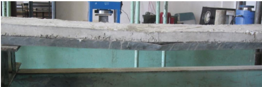
Fig. 6 Failure in hole punched specimen
