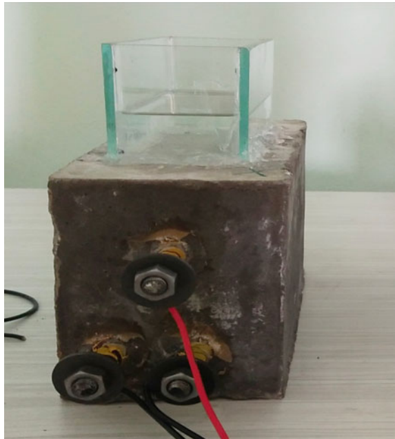
Fig. 5 Experimental setup of ASTM G 109
