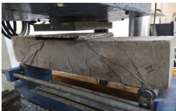
(b) Two-sided shear failure
