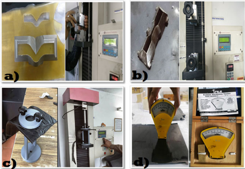
Fig. 3 a, b Mould for tensile, elongation and for tear load testing and Universal Tester Machine. c Mould for puncture resistance testing and Universal Tester Machine d Shore A Durometer
