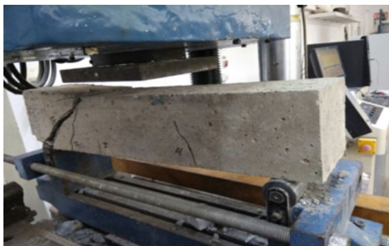
(c) One-sided shear failure
