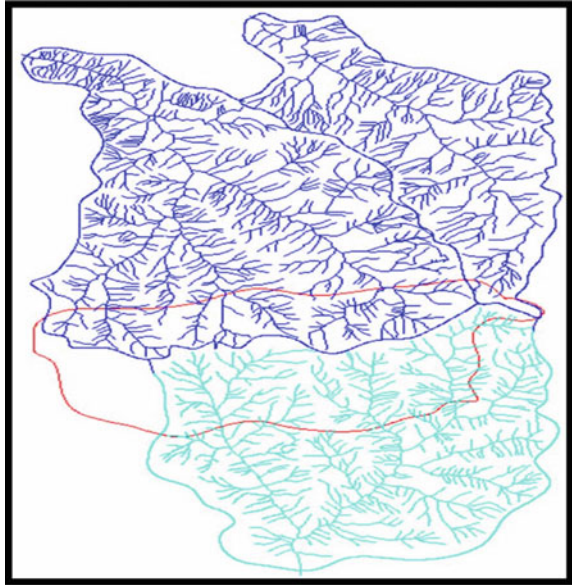
Fig. 2.2 Drainage map of Shimla city: partly in Satluj (above) and partly in Yamuna Basin (below)
