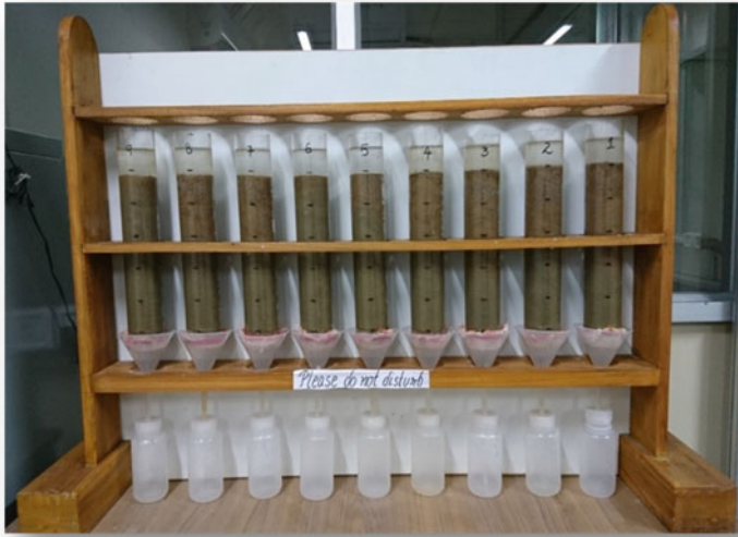
Fig. 9.1 Soil column setup used for studying the transport of nano-nutrients in the laboratory
