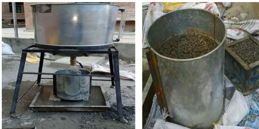
Fig. 1 Infiltrometer and sample in a specimen
