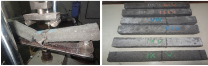
Fig. 4 Failure pattern of specimens of flexural loading
