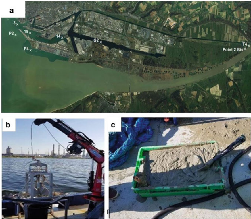
Fig. 1 a Map of investigated areas. b Dredging operation. c Homogenized sample
