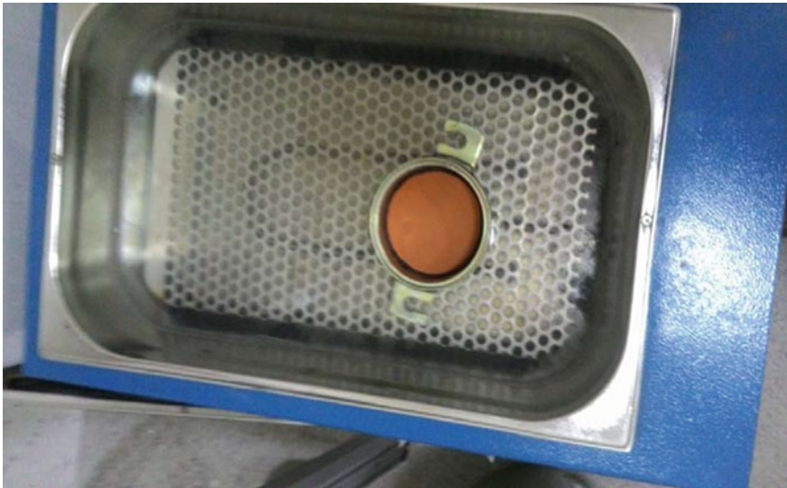
Fig. 4 Photo of marshall water tank
