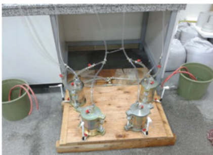
Fig. 1 OCTOPUS experiment set and the schematic diagram of falling head permeability test
