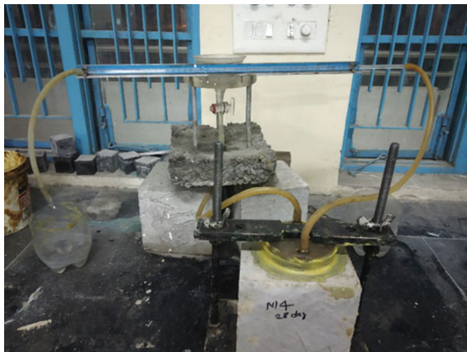
Fig. 3 Initial surface absorption testing apparatus
