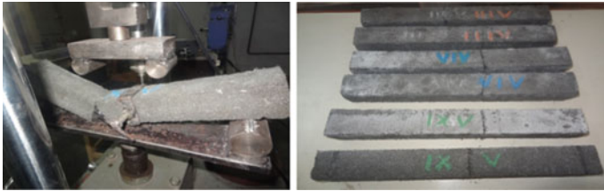
Fig. 4 Failure pattern of specimens of flexural loading
