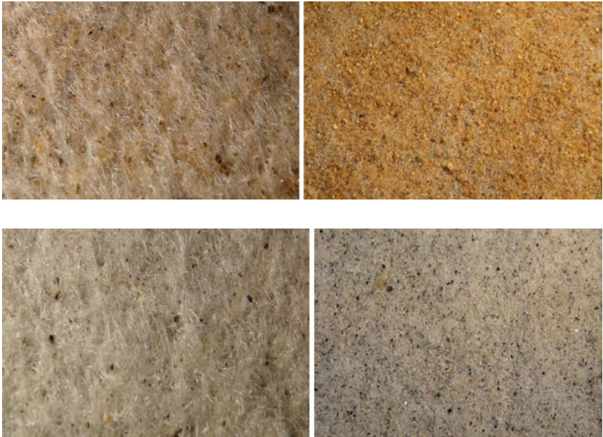
Fig. 18 a Sand-fibre adhesion in dry RS (left) and 25% water content RS (right). b Sand-fibre adhesion in dry MS (left) and 25% water content MS (right)
