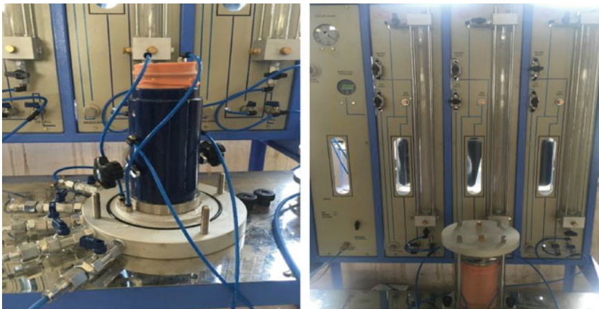
Fig. 2 a Sample under preparation b Flexible wall permeability test apparatus
