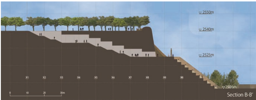
Fig. 16 Section of the staircase that connects the platform and the top of the plateau. (© Shigeyuki Okazaki/ Tokyo University of the Arts)
