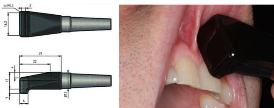
Fig. 3.17 Left: CAD drawings of prototype ultrasound probe for use on commercial clinical scanner (Mindray ZS3). Right: Photo of an in vivo scan. Note the probe geometry shown here. The transmitting and receiving surface of the probe, i.e. the aperture is transverse with respect to the probe cable. This allows the probe to enter into the oral cavity to reach the molars, where cable is required to run parallel to the tooth line to exit the mouth
