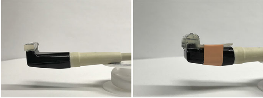
Fig. 3.19 Gel standoff for imaging superficial structures. Left: Transducer array from Fig. 3.17 with standoff pad as used in Fig. 3.15. Right: A 3D printed holder for securing the standoff pad to the aperture and preventing lateral or elevational slipping. The holder acts as a collar between the aperture of the transducer and the gel block (pad). For clinical scan an additional sheath is placed over the transducer as shown on the right to act as a barrier for infection transmission
