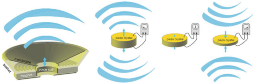
Fig. 1.1 Mechanics of generating sound and ultrasound. Left: Schematic of a loudspeaker illustrating how an electrical signal excites the magnet which then moves the cone to produce a (mechanical) sound wave. Right: Ultrasound can be generated by using a piezo crystal, whose thickness expands and contracts when exposed to negative or positive voltage, respectively (as indicated by the voltmeter)
