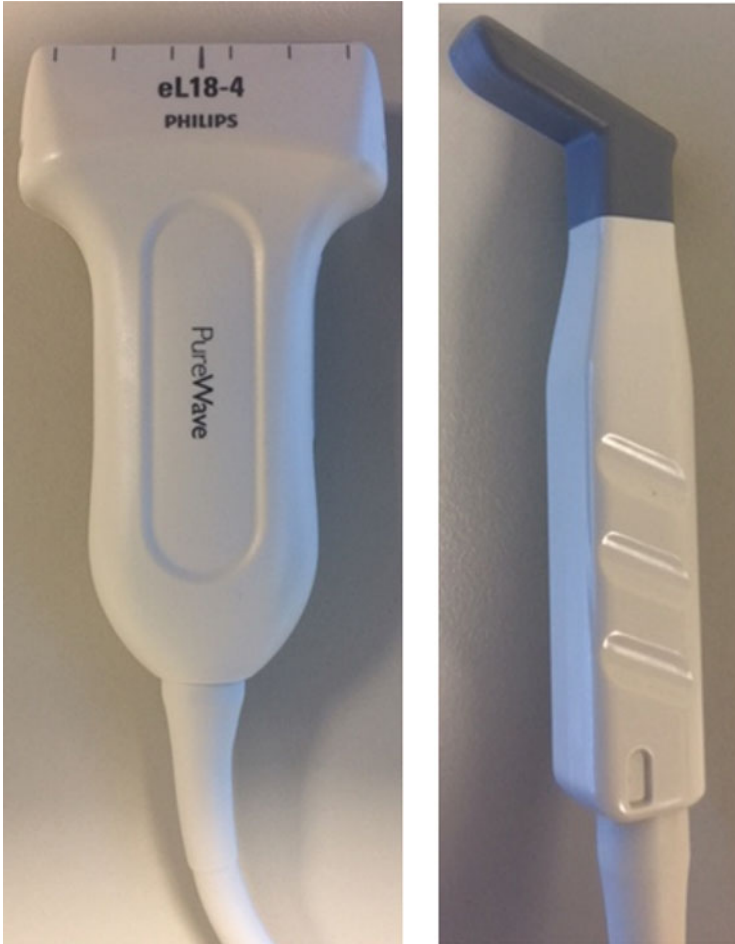
Fig. 2.2 Example of linear Philips® transducers (left-hand side is a traditional linear transducer and right-hand side is a hockey stick type transducer, which can be used intraorally on the cheek or tongue, for instance)
