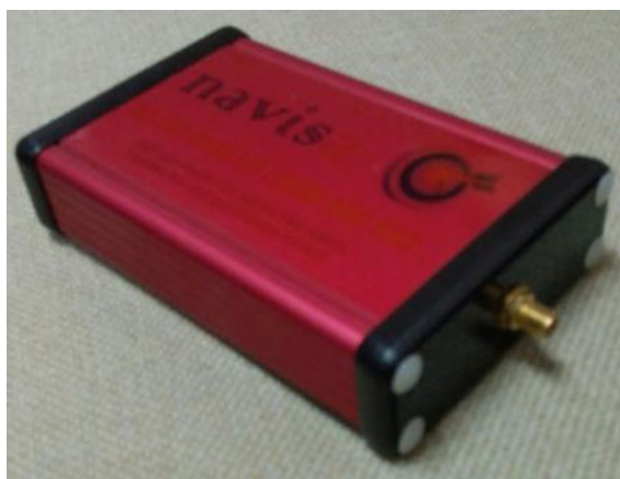
Fig. 3 GNSS receiver module of NavisA: it can be connected to an android tablet through Bluetooth or with a cable to a PC
