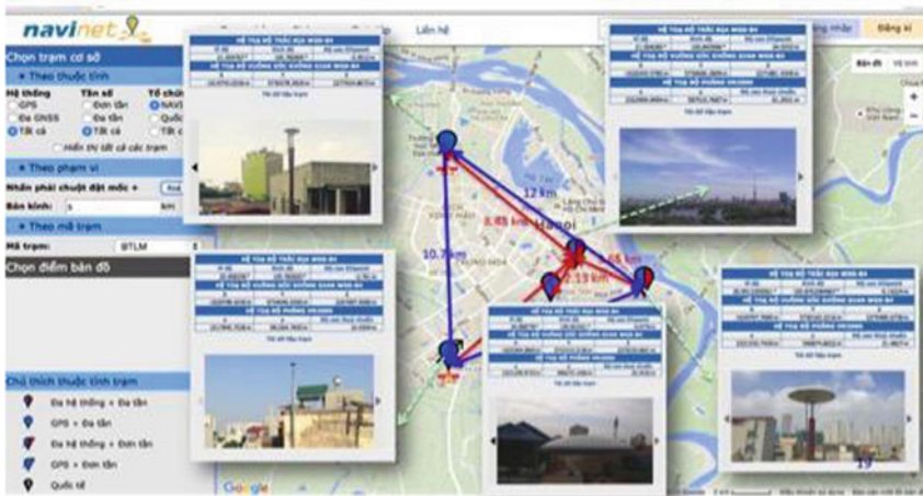
Fig. 4 NaviNet, a small-scale network of NavisA receivers to provide differential correction for precise positioning
