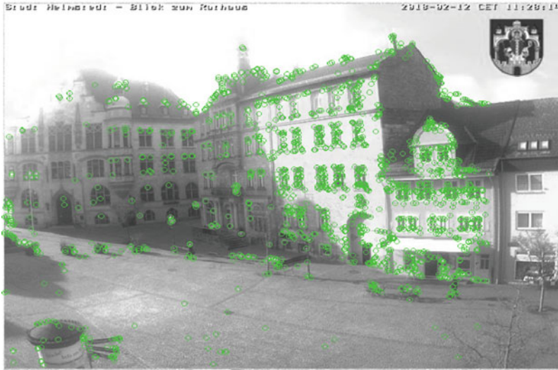
Fig. 9 BRISK applied to a BlockSee frame to extract features and reveal rototranslations of the camera FoV. Frame shot on 12 Feb 2018
