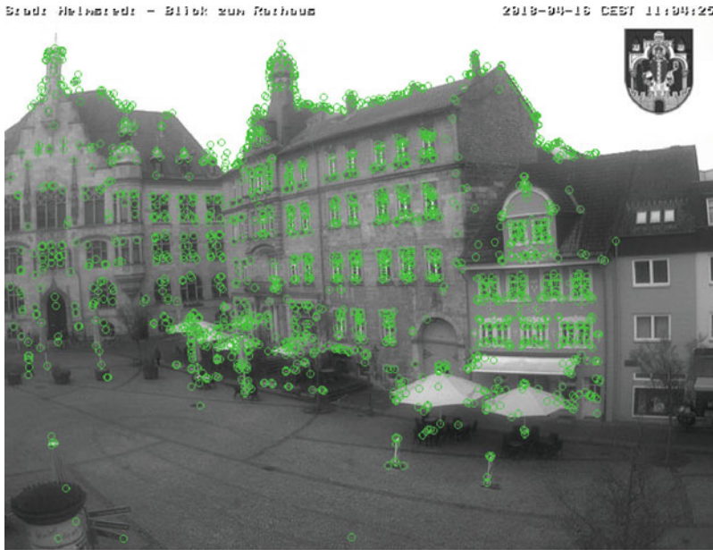
Fig. 10 BRISK applied to a BlockSee frame to extract features and reveal rototranslations of the camera FoV. Frame shot on 15 Apr 2018
