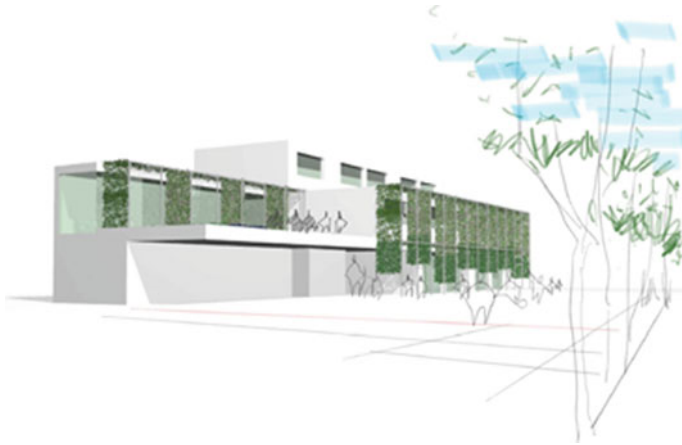
Fig. 2 School rendering with NBS implementation: East façade with green walls and roofs
