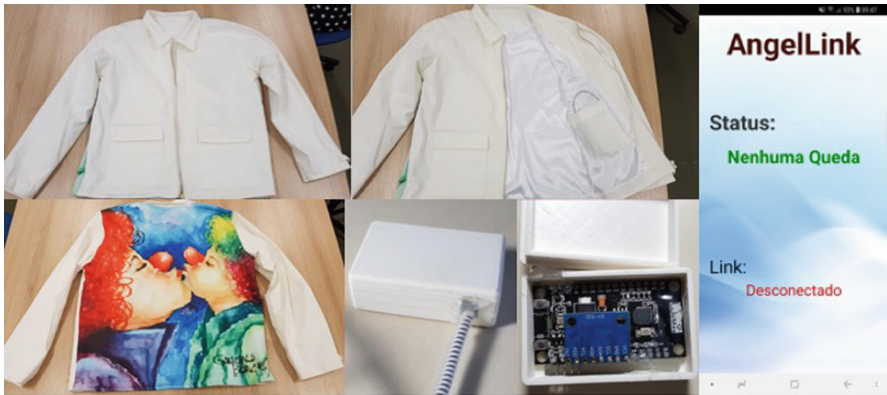
Fig. 1. Jacket equipped with falls detection system, representing the front view; the interior view (showing the pocket where the box with the device is inserted); the back view (with the print “Palhaças” by Gonçalo Borges); the 3D printed box; the electronic devices inside the box; and the application interface.
