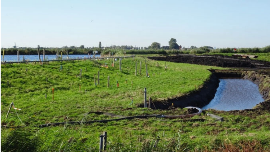
Fig. 8 View of the test site during one of the dewatering stages included in the stress test
