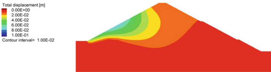
Fig. 8 First impoundment behavior—Total displacement [m]
