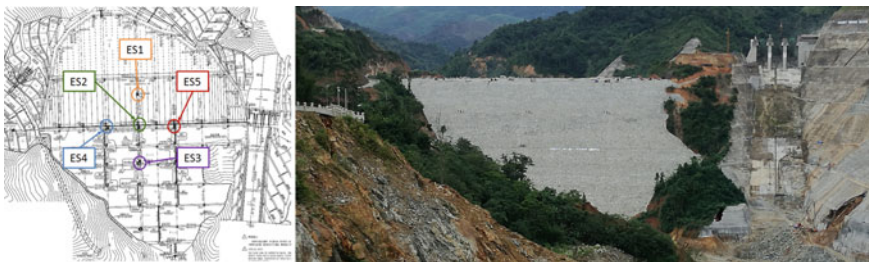
Fig. 13 Layout of the electromagnetic settlement gauges and downstream view of the construction progress in May 2019
