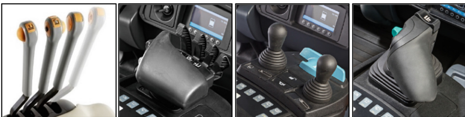
Fig. 1. State-of-the-art controls for forklift masts [14, 15]
