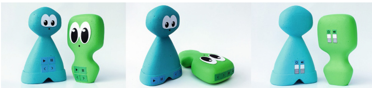
Fig. 2. Model A with buttons 1 and model B with buttons 1 (left); model A with buttons 2 and model B with buttons 3 (center); model A and model B with the graphic representation of the real buttons (right).
