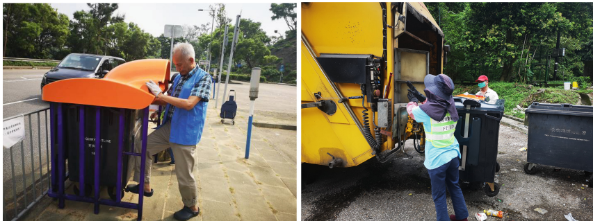
Fig. 6. Frontline cleaning workers unlocking the waste skip of the roller-fence design and emptying the two-fold waste.
