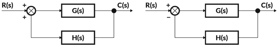
Fig. 1. Closed-loop positive (left) and negative (right) feedback systems.
