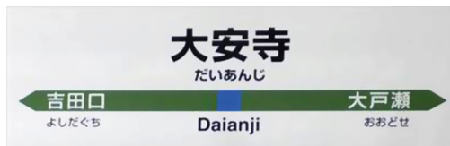
Fig. 1. An example platform display showing current, preceding and succeeding stations. This is set in outer illumination conditions.
