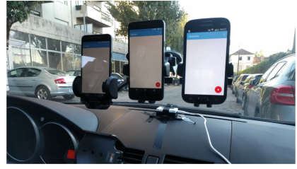
(b) Combining three smartphones and three car mounts allowed to concurrently execute two experiments
