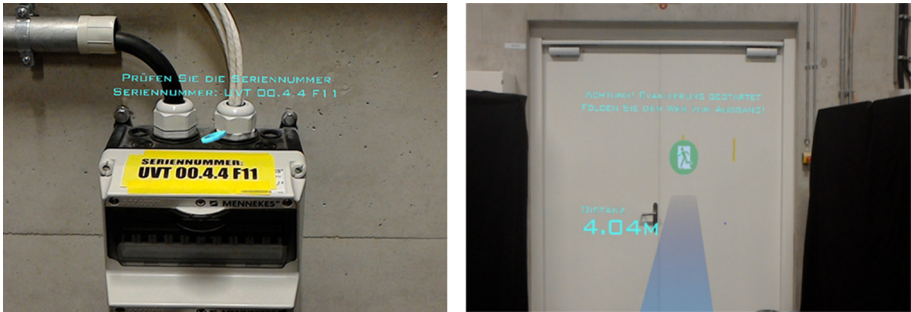
Fig. 1. Exemplary augmented reality information depending on the workers current position. Left: an instruction to check a serial number. Right: displaying an evacuation route in case of emergency.
