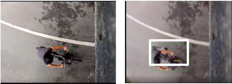
Fig. 2. Determining bounding box around the object of interest.
