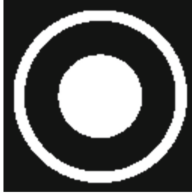
Fig. 3. A globally non- Q -convex shape that is locally Q -convex in each window position, e.g., with window size 5 \times 5 .
