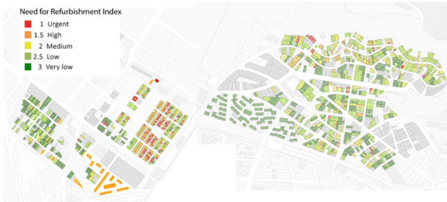
Fig. 37 Need for refurbishment index in El Bon Pastor (left) and Roquetes (right)
