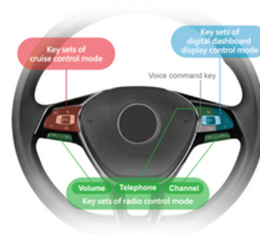
Fig. 1. Control button sets of various functions on existing multi-function steering wheel.
