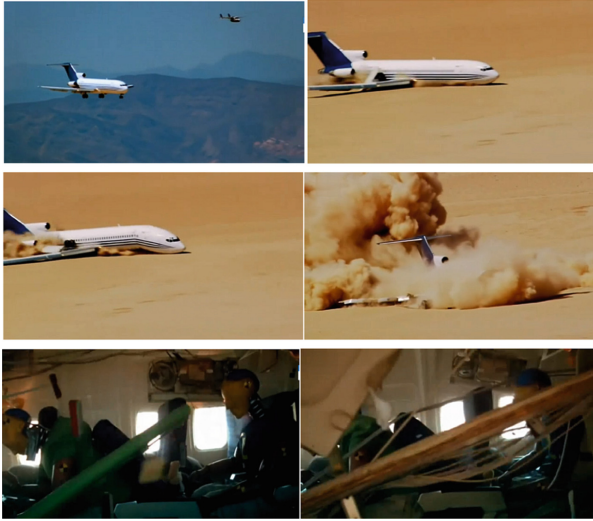
Fig. 1. Test of Boeing 727 aircraft's emergency landing
