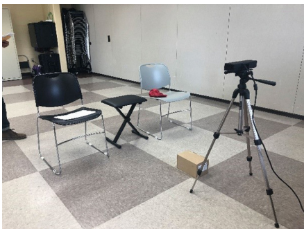
Fig. 1. The testing setup with the Microsoft Kinect.
