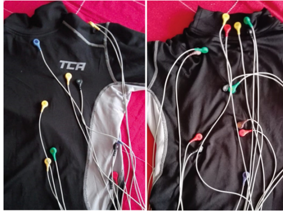
Fig. 2. Compression shirts of the patronized system, with the cables placed on the NaCl electrodes ready for the acquisition of biopotentials.
