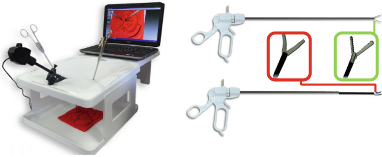
Fig. 1. Fundamental of Laparoscopic Surgery (FLS) box, connected to a computer screen, and equipped with an endoscopic grasper (green square), and scissors (red square).
