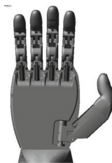
Fig. 2. Final prototype of Maki 3.0 developed at the Universidad Politécnica Salesiana [7].
