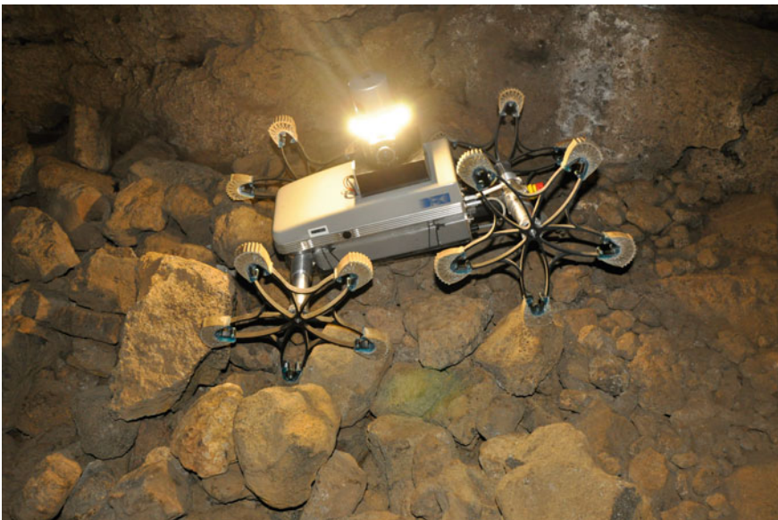
Fig. 3 The kinematically complex robot, Asguard, moving in a lava tube on Lanzarote using methods for environmental detection, model-based motion planning, and reactive control. (Photo DFKI GmbH)
