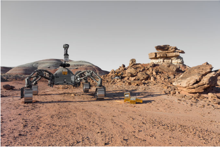
Fig. 2 The robot system SherpaTT during autonomous execution of infrastructure assembly and sample collection using modular payload modules during field testing in a desert region in Utah, USA. (Photo DFKI GmbH)
