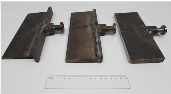
Fig. 3. Narrow dies with a thickness of 4 mm, 8 mm and 12 mm.
