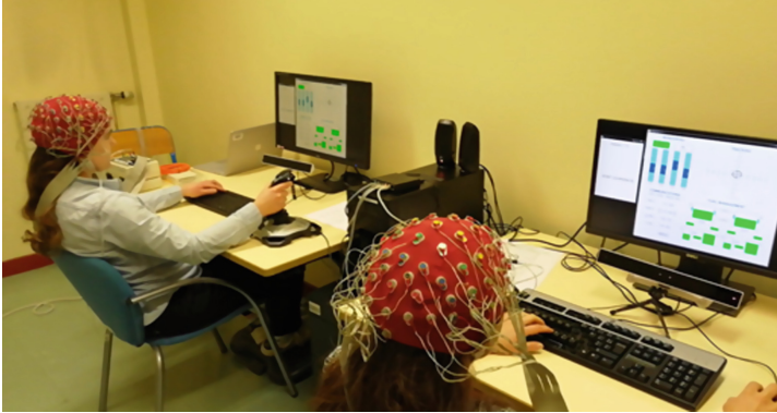
Fig. 1. Experimental setup with the two teammates equipped with a 64 electrode EEG system and performing a modified version of the MATB.
