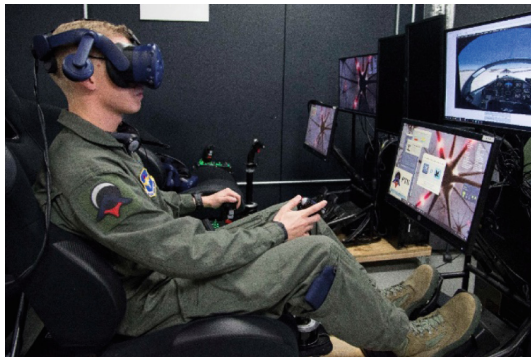
Fig. 1. PTN station: VR headset, controls, displays. (U.S. Air Force photo by Sean M. Worrell)
