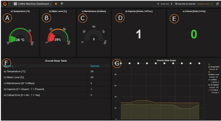
Fig. 3. Top: Dashboard showing the optimal state of the coffee machine. Bottom: Showcase of the encoding schema of the sensor data using the dashboard.
