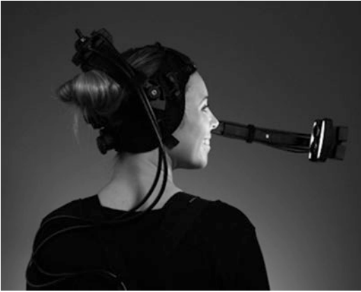
Fig. 38.7 Di4D's portable head-mounted camera. (Reproduced with permission from Dimensional Imaging Limited, © 2020)
