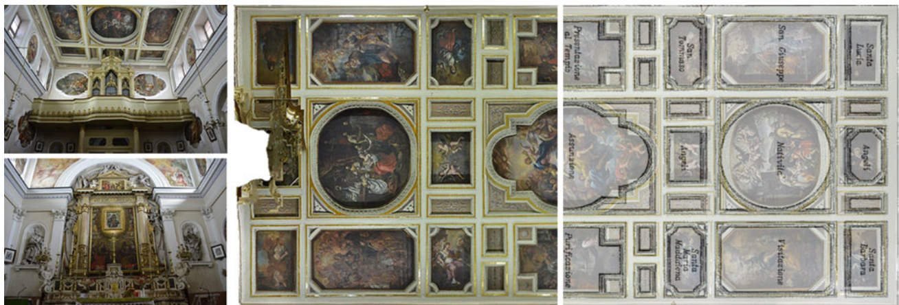
Fig. 4 On top left: the organ. Bottom left: the Baroque and Altar. On the right: orthorectified image of the wooden coffer obtained from image-based survey with SLR camera and with the software Photoscan;
