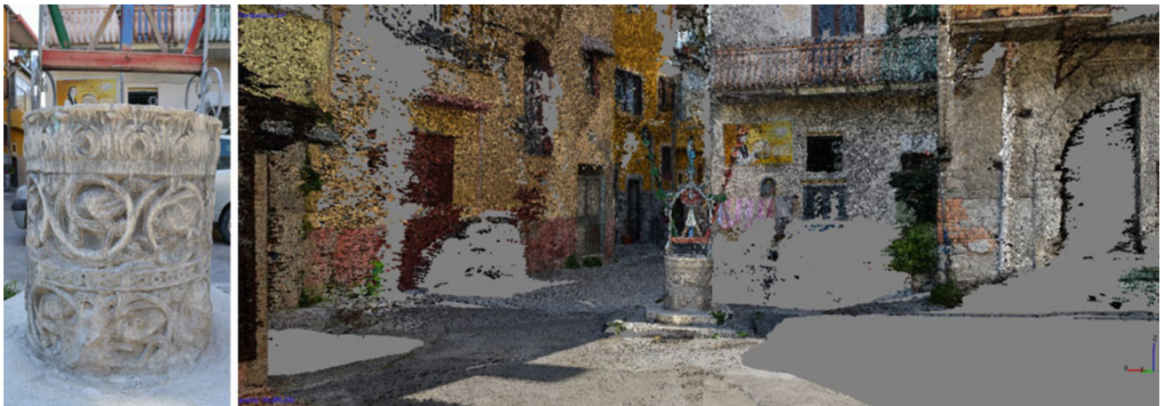
Fig. 7 On the left: Water well in the Califano courtyard, where the Tosello Madre dell'Africano is set up. On the right: The complexity of the urban space of the courtyard is rendered through a cloud points obtained with photogrammetric survey of the well
