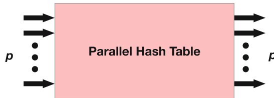
Fig. 1. A hash table that is capable of processing p operations in parallel.
