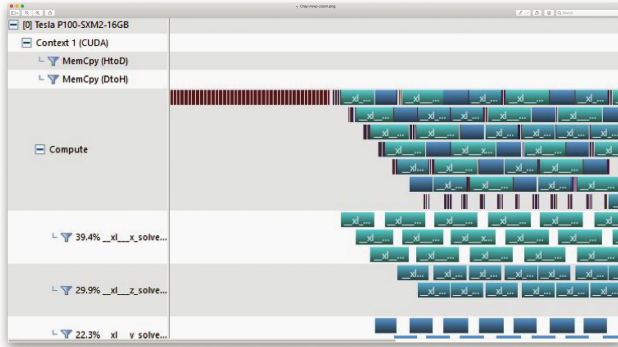
Fig. 8. Execution timeline of SP-MZ Class C on Cori GPU as seen on the profiler
