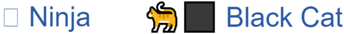
Fig. 3. A font fallback box glyph (left) and decomposed emojis (right). Emojis that cannot be represented by the user’s font file are rendered in these styles.
