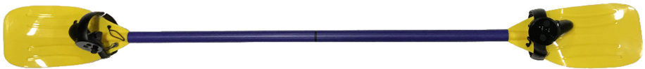
Fig. 1. The proposed “smart” paddle with the two VR controllers rigidly affixed to the two blades for 6-DOF tracking and vibration feedback when submerged in the virtual water.
