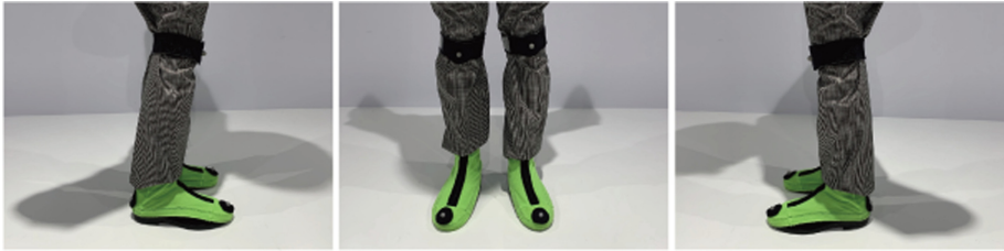
Fig. 6. Attachment locations of the reflection markers for measuring the obstacle avoidance movement.
