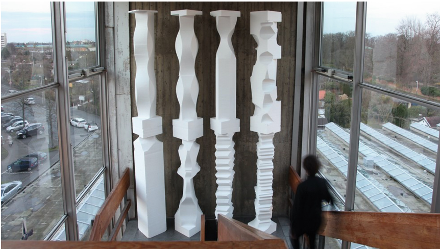
Fig. 1. Robotically hot-wire cut columns
