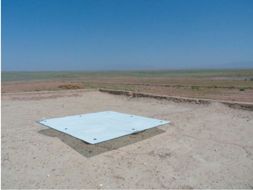
Fig. 11.3 A glass tray (100 cm × 100 cm) covered by a 2-mm PVC net mesh used for dust collection
