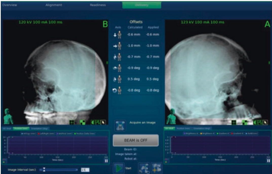
Fig. 4.3 The treatment delivery PC screen during treatment of an intracranial target. X-ray image pairs are automatically acquired throughout treatment, and the target location and orientation (i.e., 6D pose, including three translational and three rotational offsets) calculated from the most recent image pair is used to apply corrections to the treatment delivery robot so that each treatment beam
