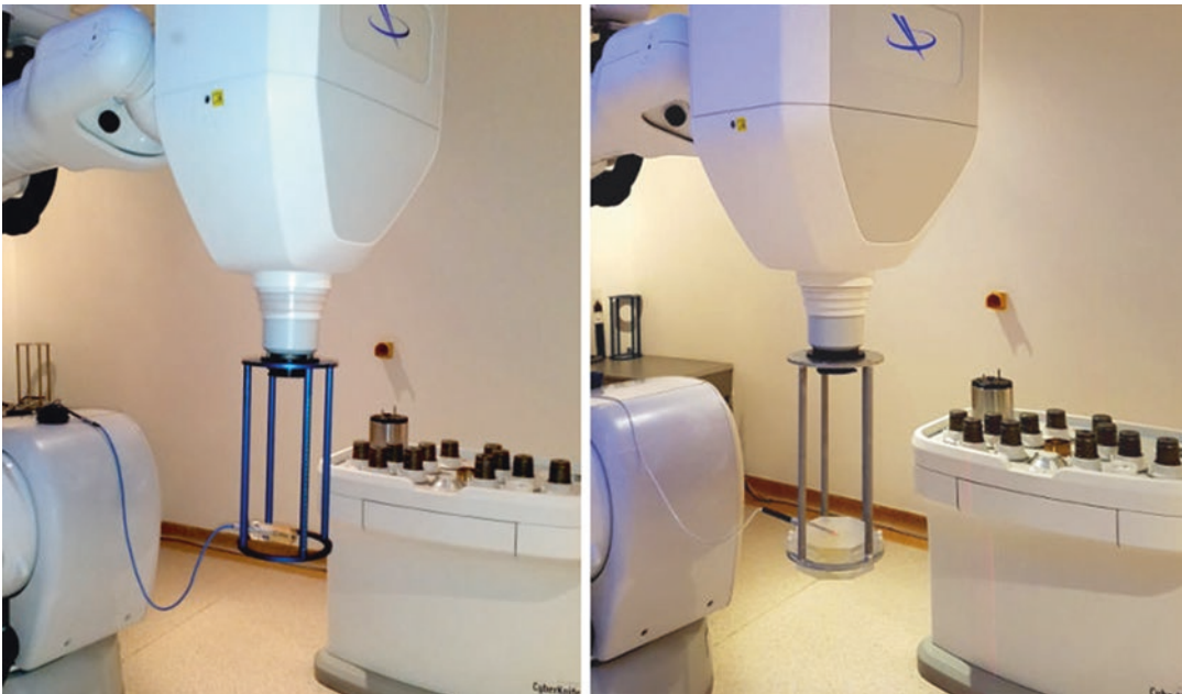
Fig. 7.3 Ion-chamber setups for daily beam output constancy measurements. On the left a classical Farmer-type ion chamber is positioned on the birdcage using a 15-mm-thick buildup cap. On the right a short cavity length
