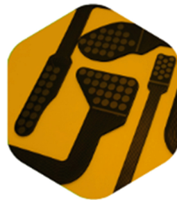
Fig. 2. HaptX skin actuators using microfluidic technology (picture created by author)
