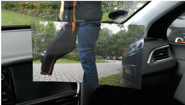
Fig. 2. An example of an AR panel in space, approximately as it will be perceived by the driver (the AR panel being transparent in our implementation).
