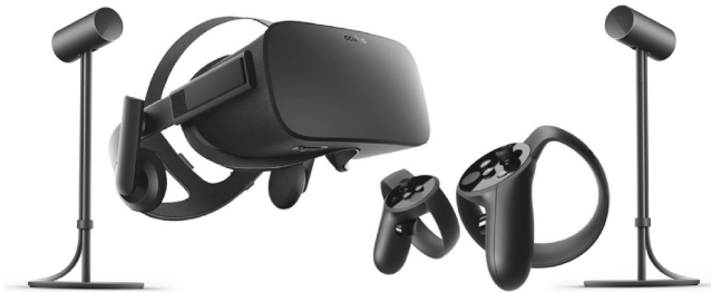
Fig. 2. Oculus Rift VR headset, Touch controllers and Constellation sensors.
