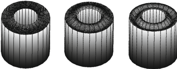
Fig. 2. The axisymmetric mode shapes of liquid vibrations in coaxial cylindrical shells.
