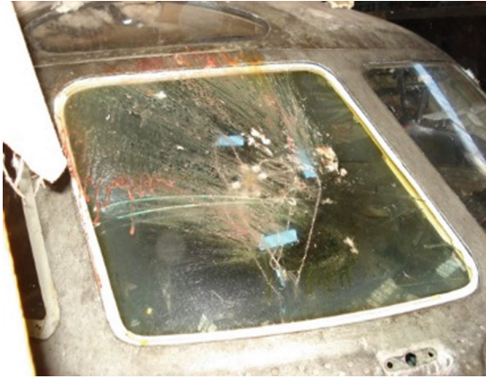
Fig. 5. Laminated glass after the strike.
