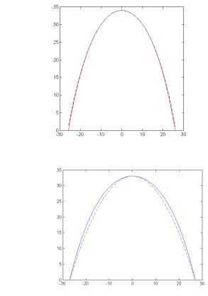
Fig. 28.2 Catenary and approximating parabola
