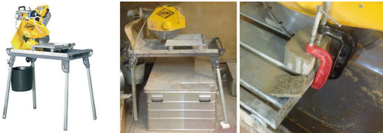
Fig. 23.3 Stone cutting machine Cedima CTS-57 G
