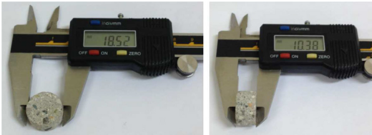
Fig. 23.2 Requirements for geometric parameters of samples
