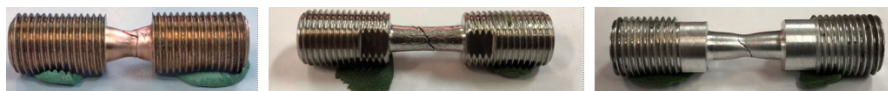
Fig. 22.6 Tested specimens: from left to right – copper M1, EP-718 alloy, aluminum alloy 1575
