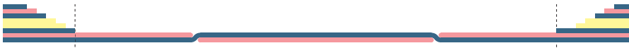
Fig. 15.7 Stacking sequence for one complete corrugation period. Dashed lines indicate transition to non-morphing parts of the design. For better visualization, the ratio between length and thickness is not to scale.
