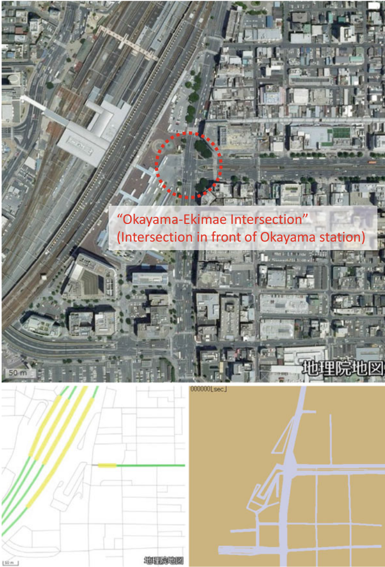
Fig. 13 Target area (top: aerial photography, bottom-left: road/tramway/railway center line map, bottom-right: simulator screen)
