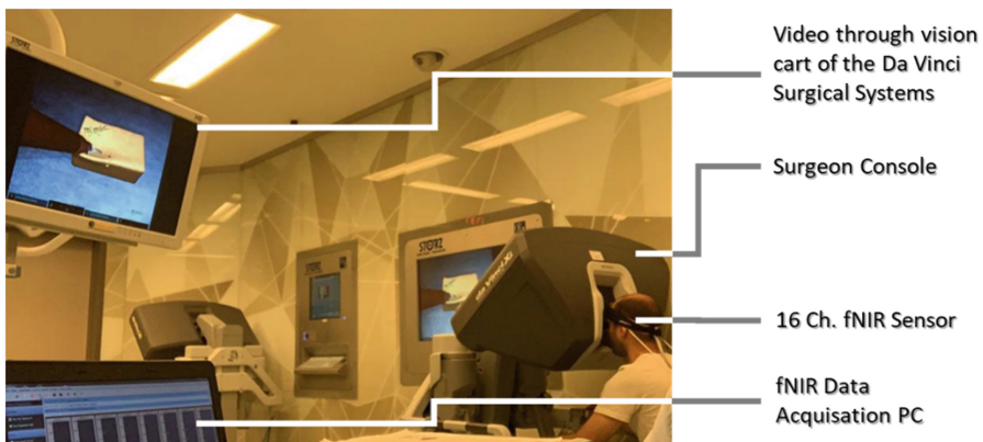
Fig. 2. A participant is performing on a task while fNIRS headband is collecting data
