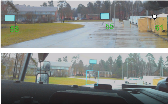
Fig. 5. Image from point of view with the AR glasses; Top: NATO symbology and distances; Bottom: alternative view with frame around object (Color figure online)
