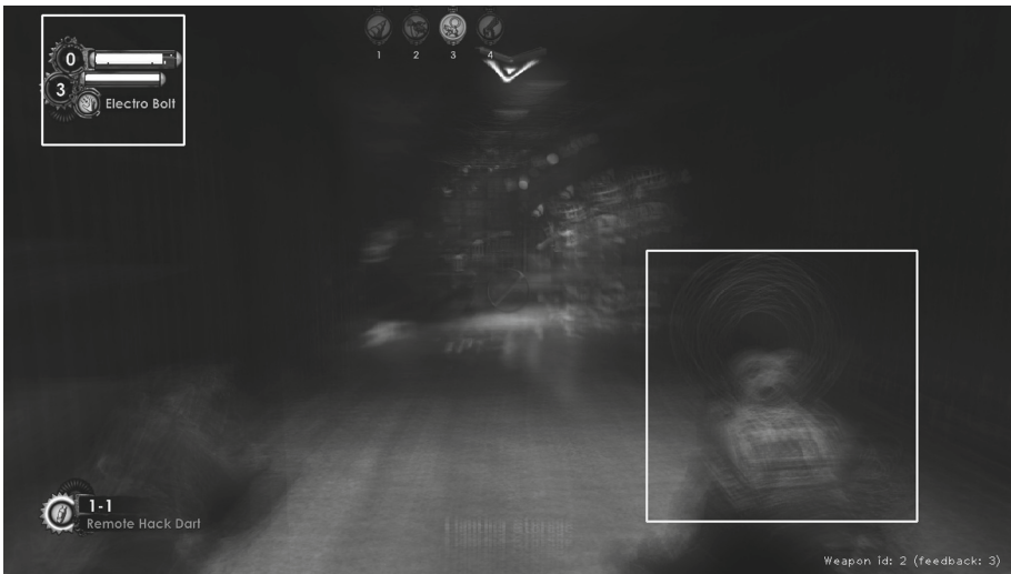
Fig. 5. Visual effect of the methods result: image from the average frame, the detected HUD area subjected to further analysis, and the identifier of the detected weapon in the lower right corner (processed frame from a screencast recorded from “Bioshock 2” [1]).
