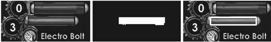
Fig. 3. Algorithm for detecting the value of the energy bar. From the left: The input area of the image detected by the classifier (additionally automatically cropped to improve processing); the image with detected pixels of proper shade and brightness (light blue); the output image with the outline of the energy bar marked, whose width is information about the energy possessed (fragments of processed frames from a screenshot recorded from “Bioshock 2” [1]). (Color figure online)
