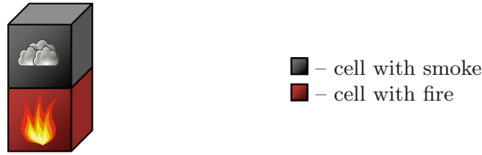
Fig. 9. Smoke release mechanism (I). Smoke is generated in the cells located directly above the cells with fire.
