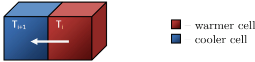
Fig. 2. Heat flow between two neighbouring cells due to thermal conductivity in the model.
