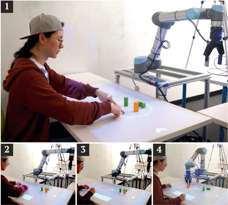
Fig. 3. PATI supports the augmented and situated specification of robot tasks, allowing users to teach their robots new tasks by directly referencing and interacting with the environment via virtual tools (e.g., shape tools) and common touch screen gestures, such as pinch, tap, and drag-and-drop. This figure illustrates a sequence of specifications for a simple pick-and-place task.
