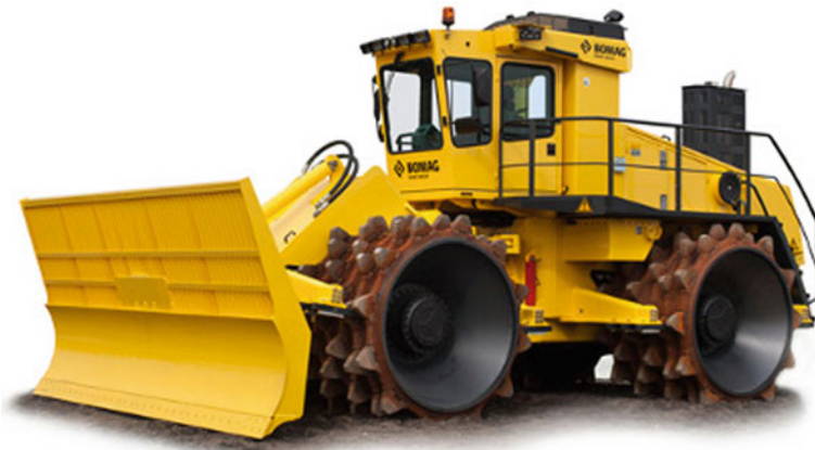
Fig. 2.31 Landfill compactor used to compact waste placed in a landfill
