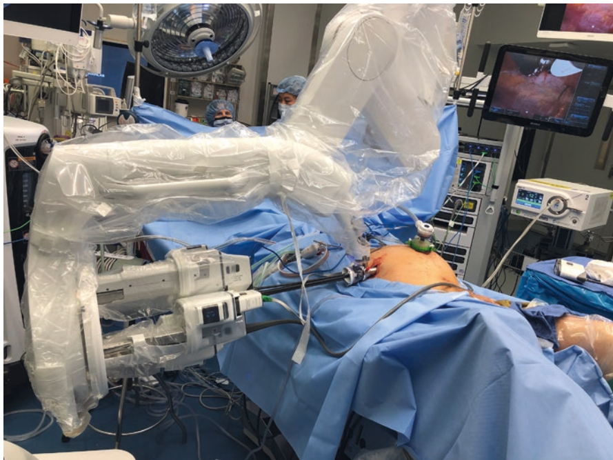
Fig. 28.3 The single port robot docked on the contralateral side of the rectus harvest
