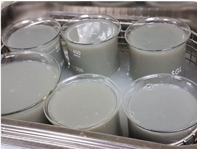
Fig. 6 Preparation of nano-PCM using ultrasonic bath
