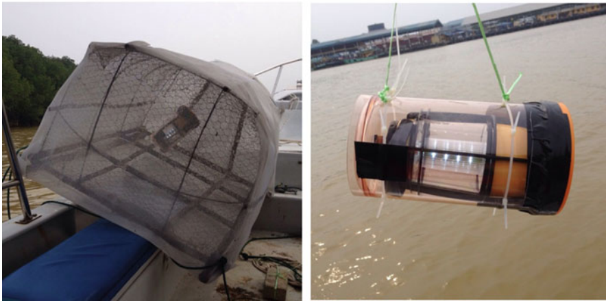
Fig. 2 Modified bubu light trap and the prepared internal light source used to attract the Ichthyoplankton during sampling
