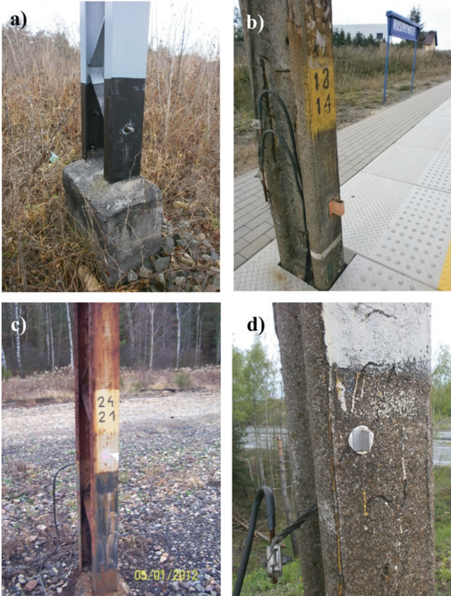
Fig. 1 Present marks of the surveying Railway Special Grid: (a) pin type (a railway line No. 661 “Dąbrowa Górnicza Towarowa DTA R5—Kozioł”), (b) box type (a railway line No. 143 “Kalety—Wrocław Popowice WP2”), (c) painted-triangle type (a railway line No. 152 “Paczyna—Lubliniec”), (d) with a T-section (a railway line No. 171 “Dąbrowa Górnicza Towarowa—Panewniki”)
