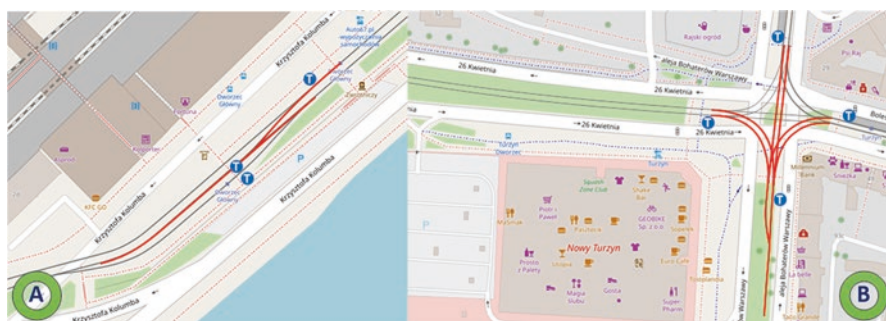
Fig. 3 The proposed use of switch-back for handling a shortened route by a bi-directional tram in Szczecin, (a) Kolumba St. (b) Boh. Warszawy/Krzywoustego intersection. (Source: Own work based on www.openstreetmap.org )
