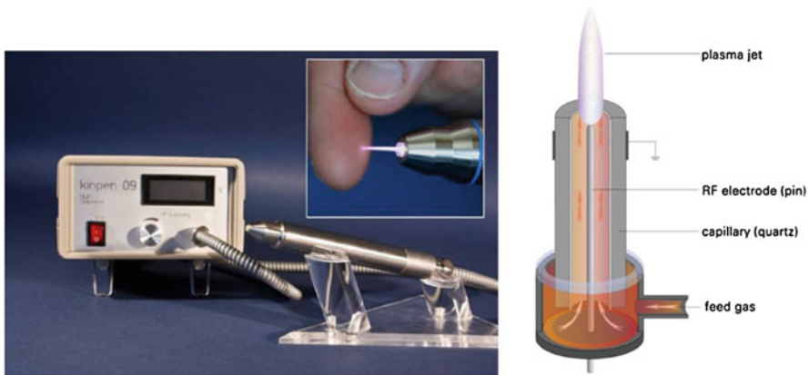
Fig. 2.12 Photo of argon APNP-J driven by RF power supply
