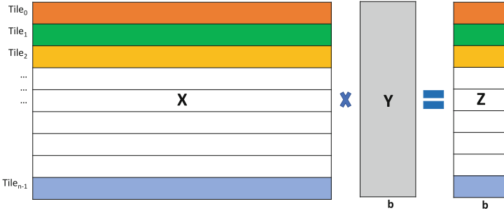
Fig. 2. Overview of tiling SpMM operation.
