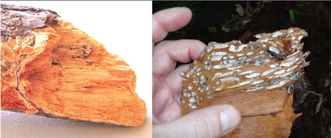
Fig. 15.4 (a) The classic stringy and bleached appearance of white-rotted wood in a hardwood. This type of decay is often colloquially referred to as “spongy white rot” or “stringy white rot.” (b) Pocket white rot in a
