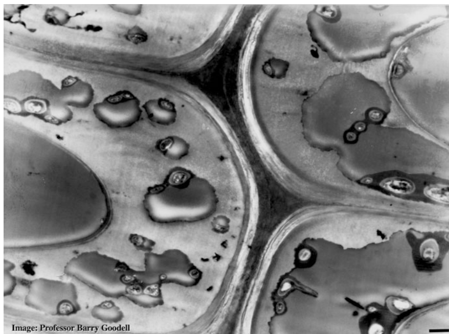
Fig. 15.6 Transmission electron micrograph of southern pine wood (xs) that was used as a cooling tower slat which was then decayed by Type I soft rot. Cavity formation shows the fungal hyphae growing within
