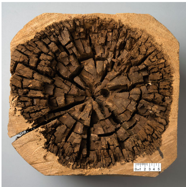
Fig. 15.3 Brown rotted wood decay from the collection of Holzforschung München, Technical University of Munich. The interior wood is in an advanced stage of brown rot degradation. At this stage, the wood is brown in color and often has a cross-hatched or cubical
